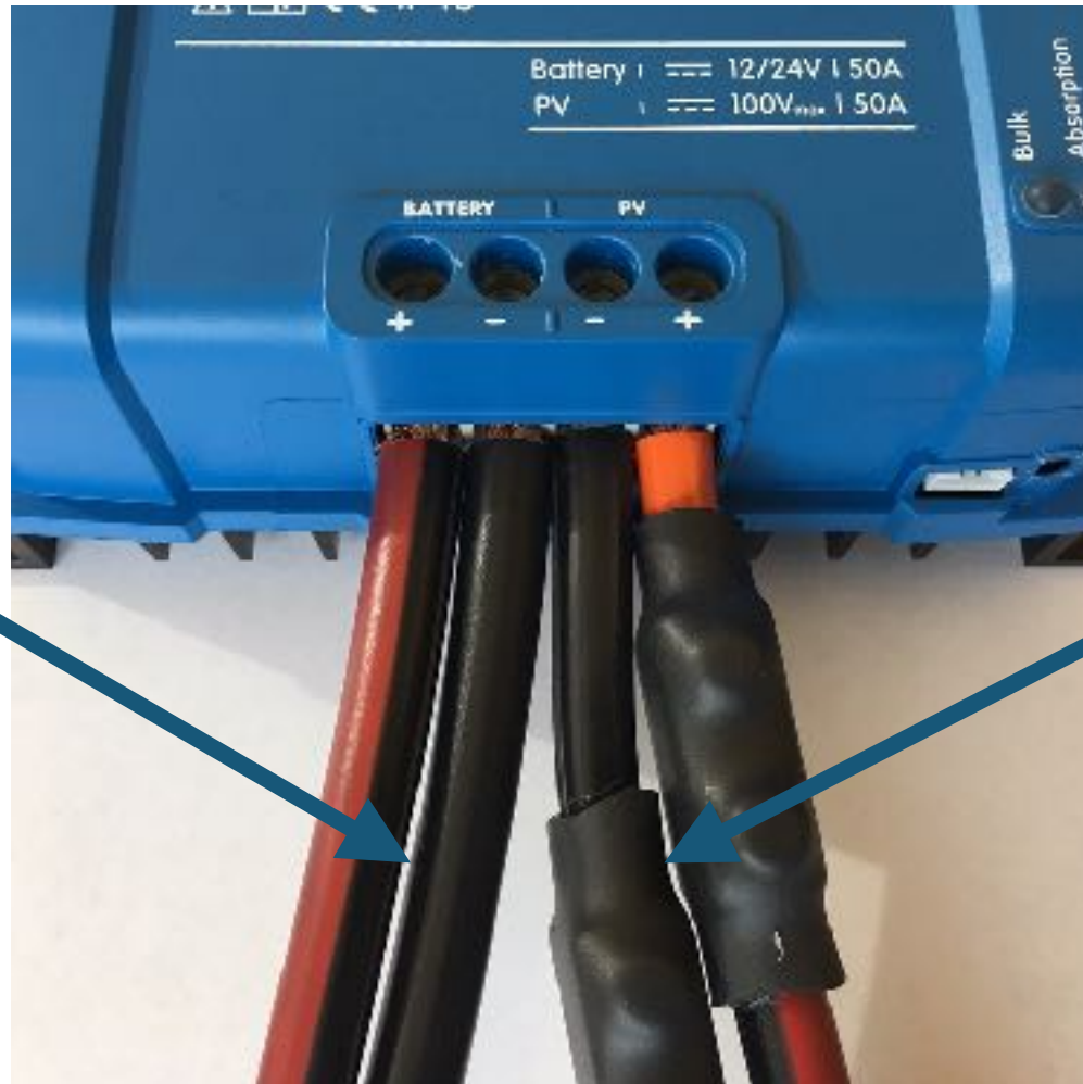
Victron MPPT 100I50 with 4ga. cable
